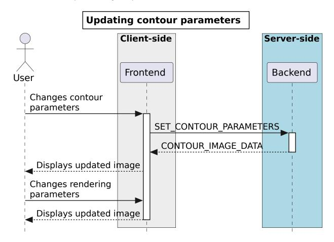
Similarly for raster images: As all the rendering is done on the frontend, any changes to the raster rendering configuration (colour map, range, scaling type) do not require any interaction between frontend and backend:
