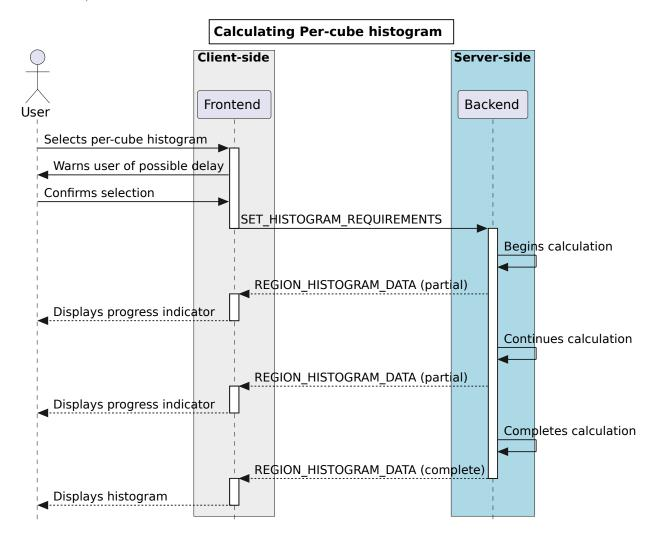
The backend should be able to cancel the histogram calculation when receiving a specific message from the frontend. By sending a second *SET\_HISTOGRAM\_REQUIREMENTS* message to the backend, with the region ID set to -2 and an empty histogram list, the frontend can indicate to the backend that the per-cube histogram is no longer required, and the backend can cancel the calculation.
